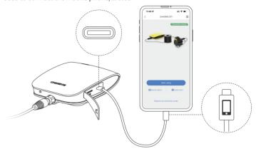
\*Note: If you cannot communicate after connection, you can turn on the OTG on your mobile phone and try to turn off WiFi and cellular traffic of your mobile phone. If you still cannot communicate normally, the mobile phone/tablet may not support the USB port function, and please use WiFi connection;
